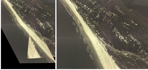
Fig. 3: Results of 4-camera virtual image composition of Matanzas Inlet (Florida) dataset (see the raw frames in Fig. 1) . when only 3 point correspondences are used. Left: The affine approach, Right: The proposed DH method.
